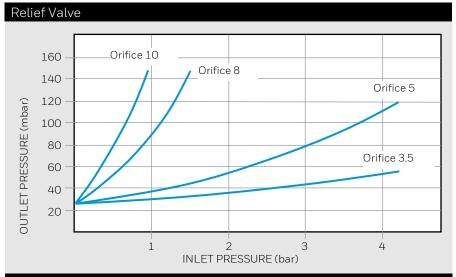
The data represented in the graph left shows the rise in outlet pressure above the set point against change in inlet pressure at a full fault situation.
