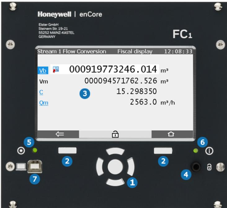
Fig. 5-1: enCore FC operation panel – example enCore FC1
