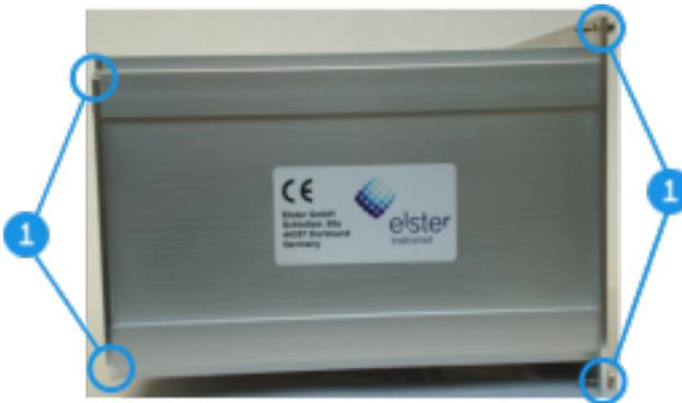
Fig. 8-1: Remove mounting screws
