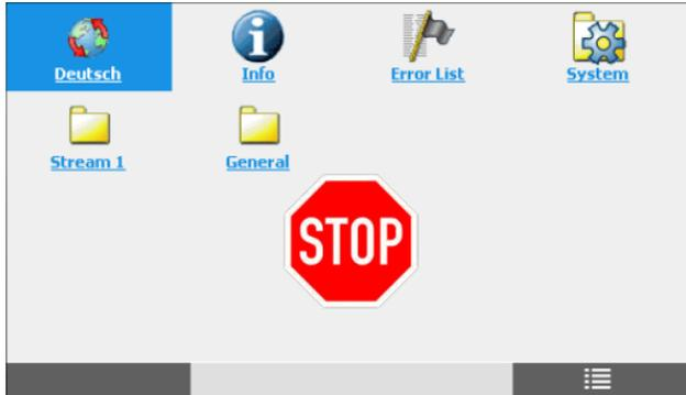
Fig. 11-4: The device signals a runtime error (stop sign).
