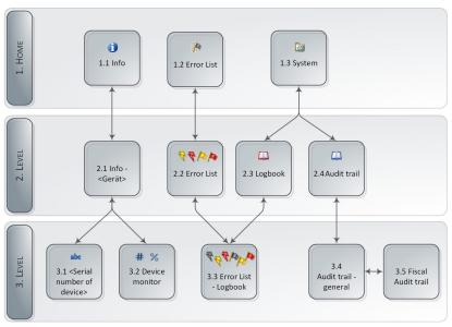
Fig. 4-1: Displays - hierarchical structure
