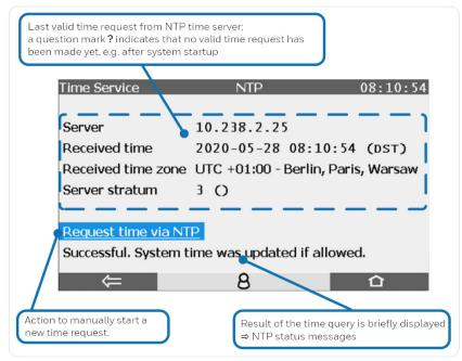
Fig. 5-9: Display NTP - example
