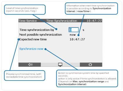
Fig. 5-6: Display Time synchronization - example
