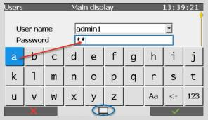
Fig. 9-7: Remote operation panel active – The **a** key has been pushed
