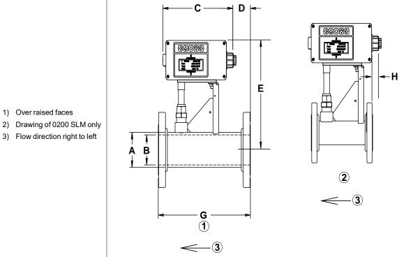
Dimensions in millimeters unless stated otherwise Approx. Nominal Model С Е А В D G Н weight size kg 0200 SLM 51 277 60 51 231 202 18 9 -0300 SLM 76 89 277 15 76 231 58 305 -0400 SLM 102 114 99 231 135 277 406 22 -0600 SLM 152 168 152 231 287 300 610 38 -
