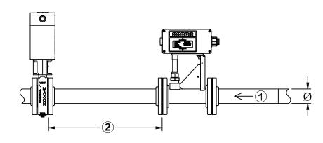
Combustion blower outlet with control valve
