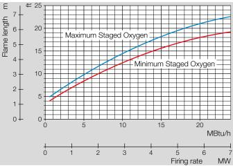
Flame lengths shown are typical for burners sized and operating at maximum design conditions. Flame lengths per unit of heat input will vary from these values when burners are operated below maximum design.
