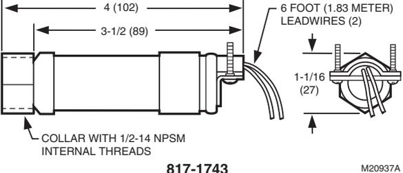
Fig. 4. Ultraviolet detector, mounting dimensions in inches (mm).
