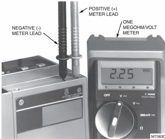
**Fig. 24. Flame signal measurement.**
