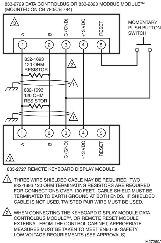
**Fig. 9. Wiring the Data ControlBus™ Module with Remote Keyboard Display Module.**
