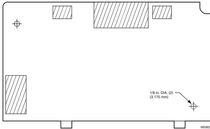
**Fig. 26. Flush mounting of a Keyboard Display Module template.**
