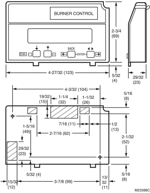
Fig. 2. Mounting dimensions of Keyboard Display Module, in inches (mm).
