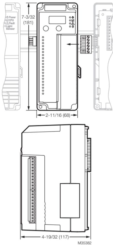
Fig. 1. Dimensions in in. (mm).
