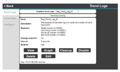
It is a good idea to activate monitoring for values that are critical for your particular application and review the behavior of these values periodically. It can help to detect longterm changes in the system or process being controlled.
