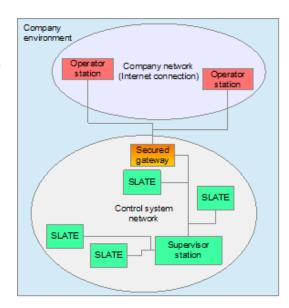
A possible example of such a secure gateway would be a typical VPN setup with a strictly defined set of approved users.
