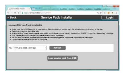
Press "Load service pack from USB" button to initiate the installation process. Please note that installation cannot be cancelled once started. Never reboot the unit during installation if not prompted to do
