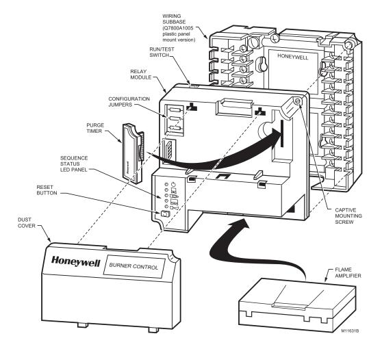
Fig. 4. 7800 SERIES Relay Module exploded view.
