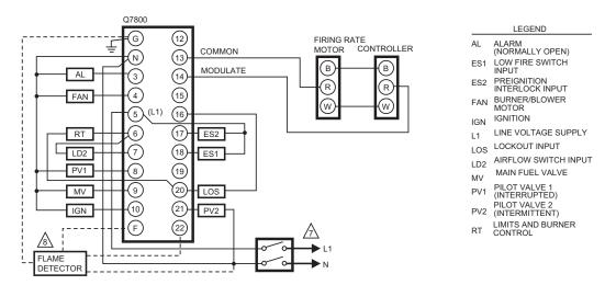
EC7820A Atmospheric + Fan Relay Module with Option for Modulation
