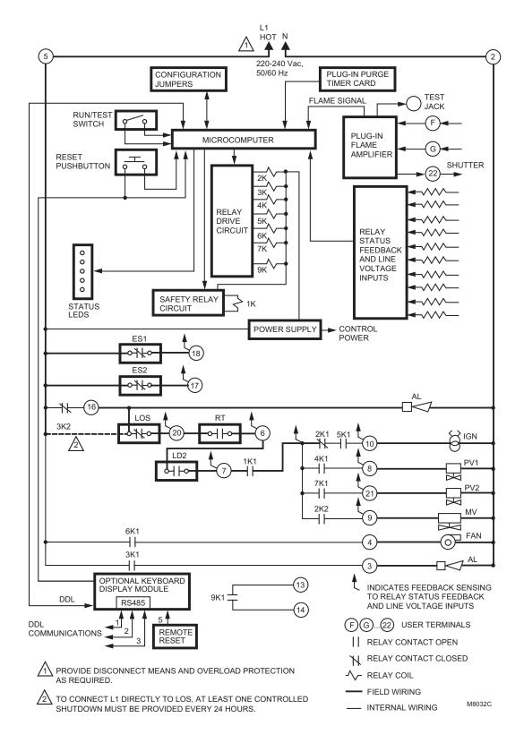
Fig. 2. Internal block diagram of EC7820A Relay Module (see Fig. for detailed wiring instructions).
