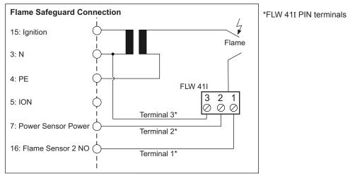
NOTE: See Figure 9h-4 (page 110) for complete wiring of FLW 41I
