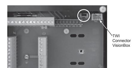
Figure 4.2 Type 3 Parameter Switch Location
