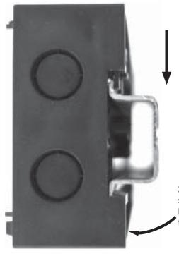
1. Push the base downward to compress the springs.
