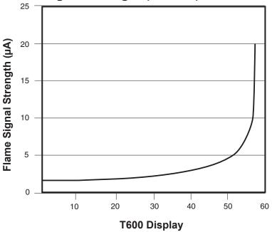
The quality of the flame signal is displayed for flame detector 1 as a number between 0 and 58. Evaluation of the flame signal is only possible with ionization flame monitoring. When using the UV 42, the maximum value is always displayed.
