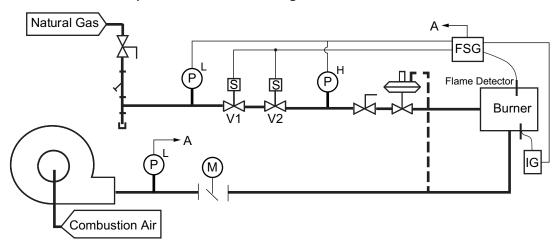
After the burner start signal, the fan is switched on and the air pressure is checked by the pressure switch. After the pre-purge time has lapsed, the ignition is switched on and the two valves V1 and V2 are opened together. See section 5, "Operational State Overview" for details on the complete sequence.
