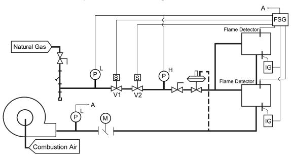
After the burner start signal, the fan is switched on and the air pressure is checked by the pressure switch. After the pre-purge time has lapsed, the ignition is switched on and the two valves V1 and V2 are opened together. On failure of either flame detector, both V1 and V2 are closed and both burners are shut-off. NOTE: Dual burner pilot ignition is also possible. See section 5, "Operational State Overview" for details on the complete sequence
