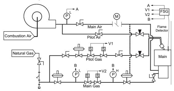
After the burner start signal, the fan is switched on and the air pressure is checked by the pressure switch. After the pre-purge time has lapsed, the ignition is switched on and the pilot valve(s), V1, is opened for the trial for ignition. After proof of pilot flame, the main valve(s), V2, is opened. See section 5, "Operational State Overview" for details on the complete sequence.
