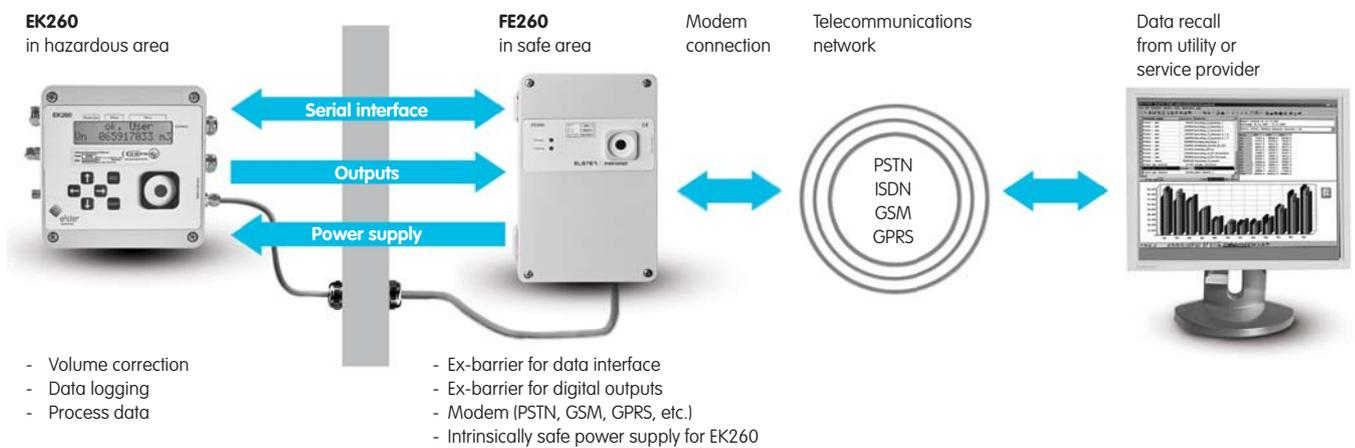
The Ex-barrier of the serial interface and the pulse outputs of the volume corrector is provided by the FE260 function extension
