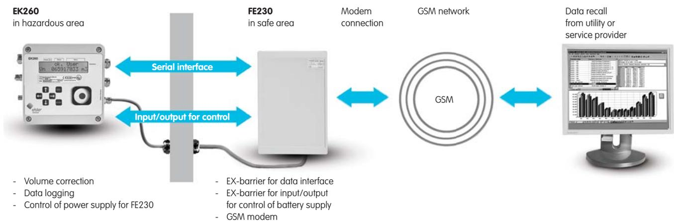
The FE230 function extension unit is a battery-operated GSM modem which allows data communication without external
