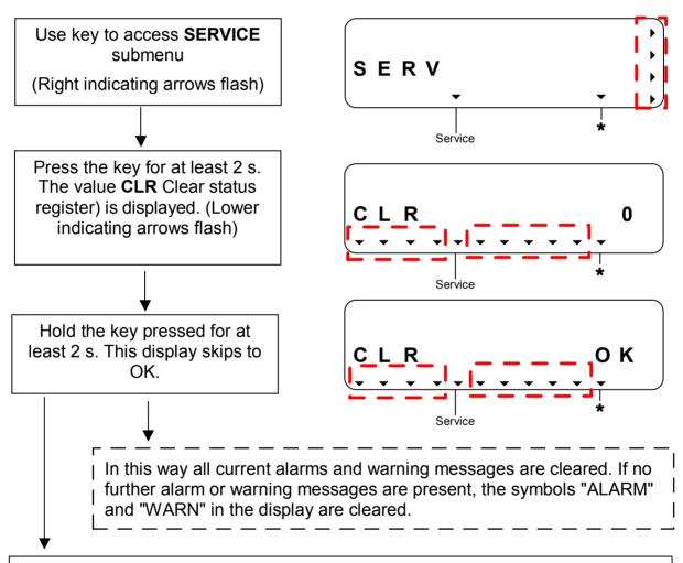
To **quit the submenu**, a value which cannot be edited is brought into the display  $(\rightarrow 2.3.2)$ . E.g. keep pressing the key until the **display test** is shown. The submenu is left by pressing the key for at least two seconds. The submenu is also left when the display switches off (after two minutes).
