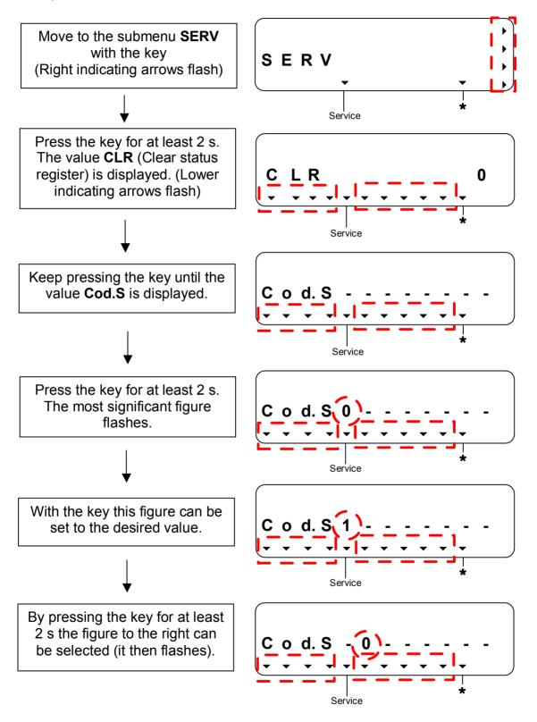
With the key this figure can be set to the desired value.
