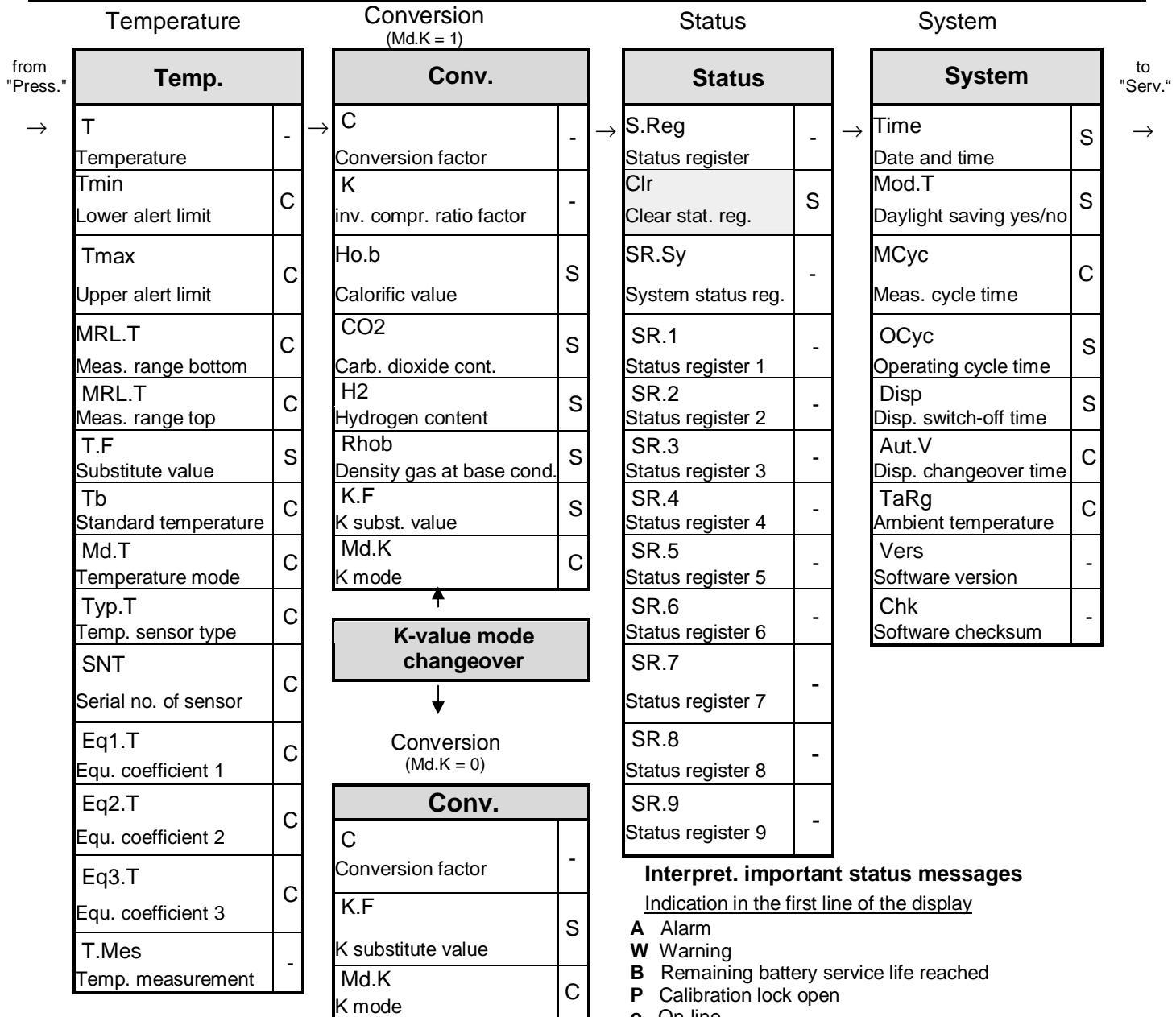
A flashing device status signals a prevailing message, a steady device status a message no longer prevailing, but which is still present in the status register. The status register "**S.Reg**" logs all alerts and warnings since the last "clear". Momentary statuses and reports can only be read via WinPADS.
