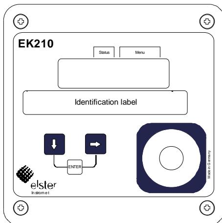
If any key is pressed, the display is activated and the present counter reading V<sub>b</sub> (volume at base conditions, predecimal places) is displayed in the User menu. All other data associated with the volume at base conditions can be displayed by pressing the keys  $\rightarrow$  (1x) and  $\downarrow$  (see second column "Standard volume" in the operation overview to these instructions).
