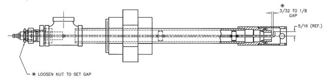
Figure 4. Replacement Electrode Bending Details
