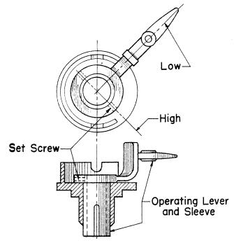
Figure 1. Drawing of the air nozzle control lever showing the set screw locations.
