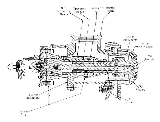
Figure 4. Cutaway View Of The 780 Seires Burner Assembly Showing The Individual Components.
