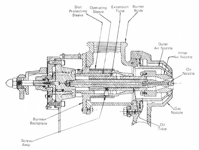
Figure 5. Cutaway Showing Burner Components
