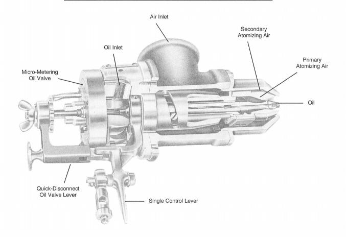
Figure 6. Sectional View Of Burner
