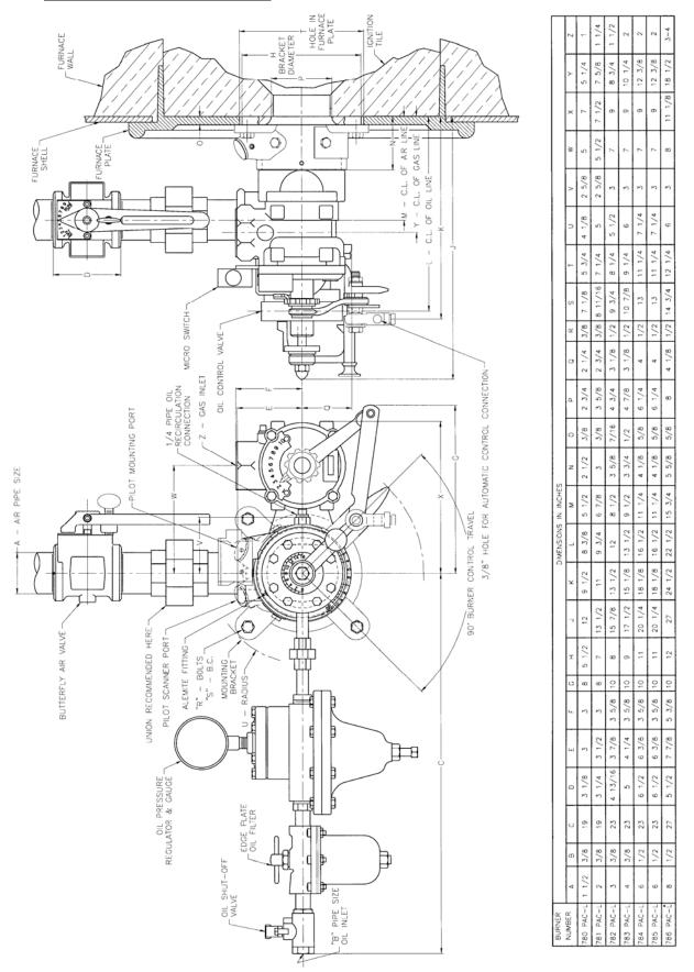
Figure 3. Dimensions - Burner With Combination Access Bracket
