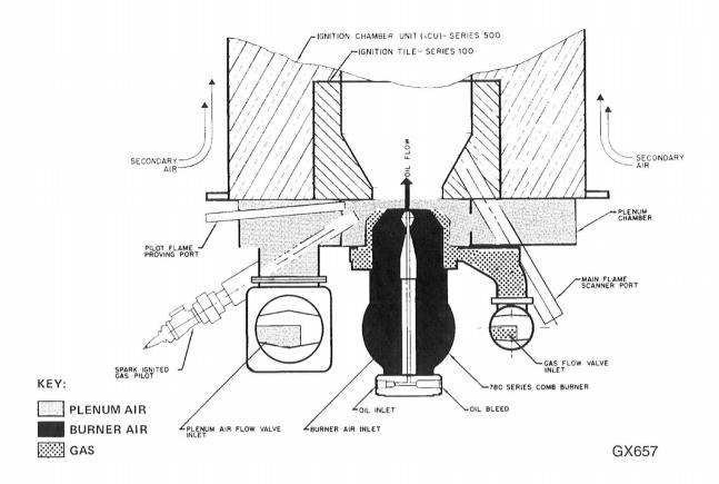
Figure 1. Flow Diagram, Wide Range Burner Unit
