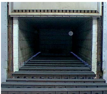
Fig. 6: Bogie hearth furnace with BIC high-speed burners
