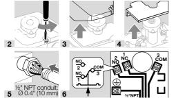
→ C6097A: The NO-to-COM connection is interrupted if the pressure drops (contacts 3 and 2 open).
