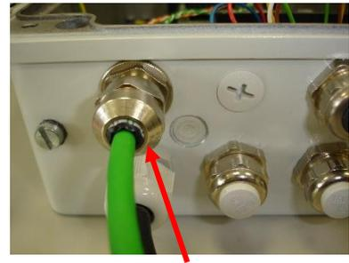
Fig. 17: Fitted EMC cable gland
