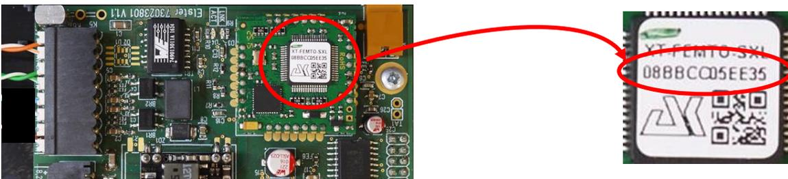
Fig. 20: MAC address of the iCE260-Ethernet
