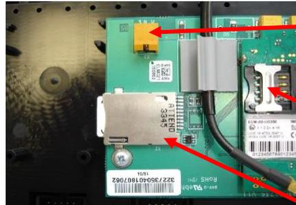
Connector for modem battery **or** internal power supply.
