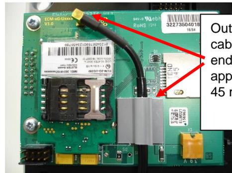
Outlet of the cable grip to end of plug is approx. 45 mm!
