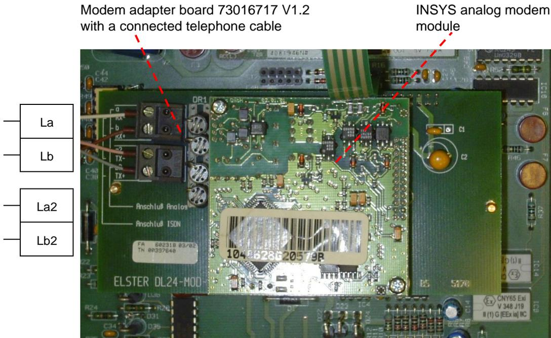
Fig. 12: INSYS Analog modem module in the FE260
