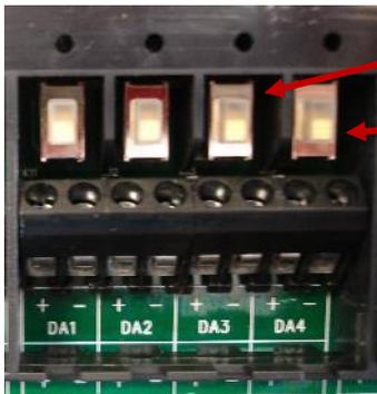
Four switches for electrical isolation for each output
