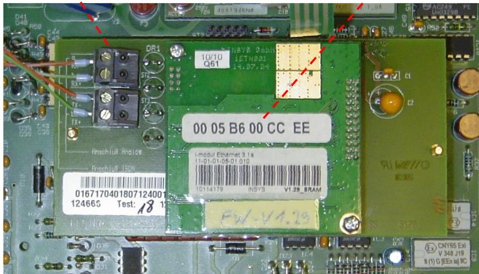
Fig. 13: INSYS Ethernet adapter in the FE260
