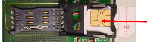
Fig. 10: SIM card slot on the ECM-GW120 modem
