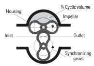
Working principle of rotary gas meters
