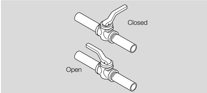
Make sure that the handle of a gas cock is at a right angle to the valve body when the valve is in the closed position. This is an important position indicator.
