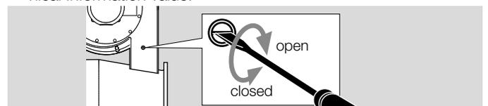
→ A pressure tap is open when the screw inside the tap is unscrewed approximately half a turn.
