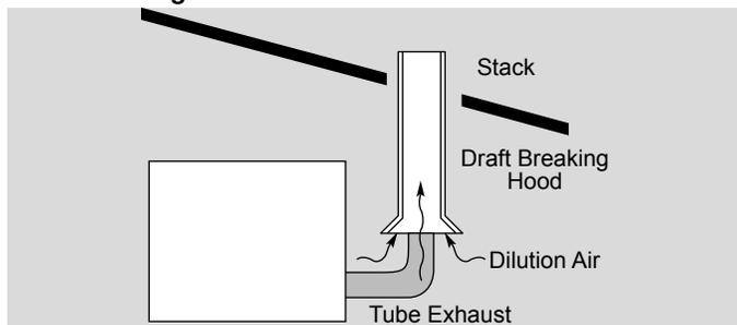
A draft breaking hood is an open connection between the heater tube exhaust and the exhaust stack. It allows fresh dilution air to pass into the exhaust and mix with the exhaust gases.
