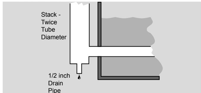
**NOTE:** Regardless of the exhaust design, pitch the immersion tube down towards the exhaust so condensate will not collect at the burner.
