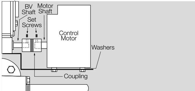
→ Be sure the control motor shaft and air butterfly valve shaft are aligned properly. If using an Eclipse Actuator Mounting Parts Kit, the supplied washers may be used as shims (stacked 0, 1, or 2 high) to ensure proper alignment. Additionally, a flexible coupling can be used to handle minor misalignment.
