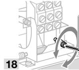
→ Turn the screw with an Allen key until the switch is actuated with the required stroke:
