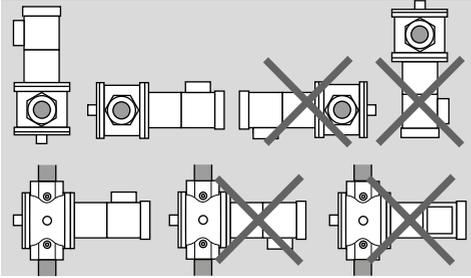
→ The motorized valve for gas VK must not be in contact with masonry. Minimum clearance to the side: 20 mm.
