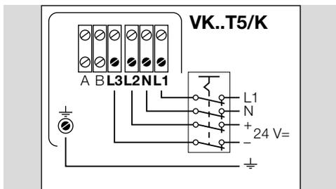
→ On VK..T5/K: in order to close the valve, both power supply points must be switched off.
