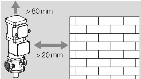
→ Ensure that there is sufficient space for installation and adjustment. Minimum clearance to the top: 80 mm.
