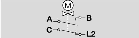
→ C-L opens as soon as the motorized valve starts to open.
