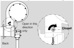
The minimum opening angle (S4) of the butterfly valve is set as follows at the factory:
