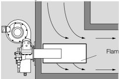
The flame tube is positioned around the burner tube and the flame. The diameter of the flame tube should be around 3 x the burner tube diameter. The length of the flame tube must cover the full length of the flame, see Technical data, page 11 (10.2 Flame length).
