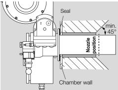
If the burner is used in heat exchangers at low temperatures, it can be installed directly on the combustion chamber. There is no need for a refractory lining. If the chamber insulation extends beyond the nozzle position of the burner, cut the insulation at the end of the burner tube at an angle of at least 45°. Detailed information can be found in the RatioMatic operating instructions at <a href="https://www.docuthek.com">www.docuthek.com</a>.
