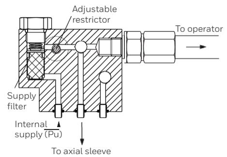
As the operator opens, a flow and hence pressure drop is created across the restrictor. The pressure drop is transferred directly to the back of the axial sleeve.
