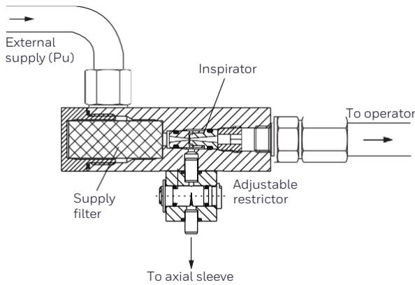
As the operator opens, a flow and hence pressure drop is created across the inspirator. The inspirator boosts the pressure drop to the back of the axial sleeve by approximately 3:1.
