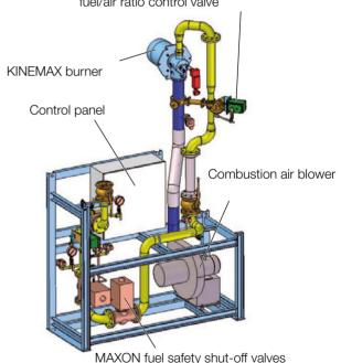
KINEMAX® Size 4 gas only burner in a complete system with burner control panel and natural gas pipe-train, including MAXON fuel safety shut-off valves and MAXON gas/air ratio control valve.
