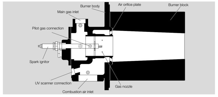
Combustion air enters the burner body and is swirled out into the burner block through the internal air orifice plate. Low pressure gas enters the burner body and exits to the block through machined ports in the gas nozzle.
