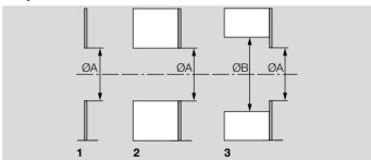
**Sketch 1:** sheet metal combustion chamber/furnace without internal insulation. Flange/opening internal diameter shall be  $\emptyset A$ .
