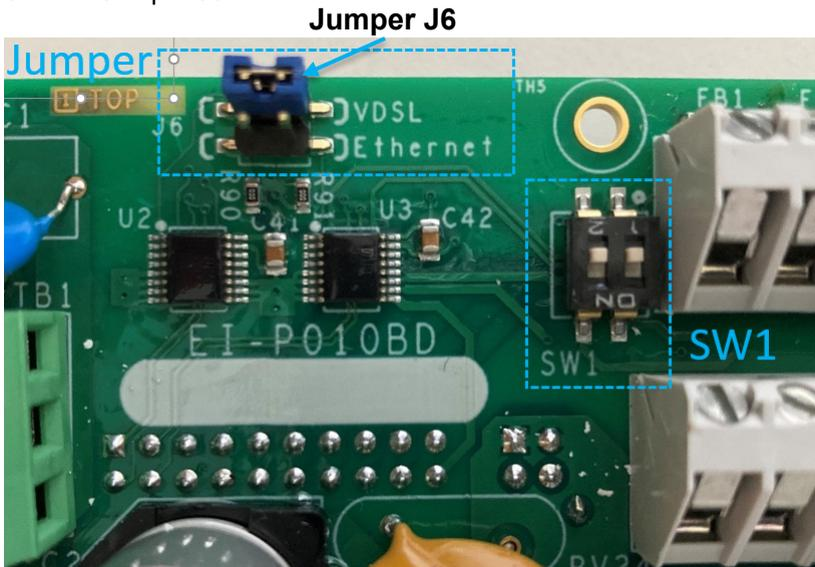
Fig. 6-1: Field Terminal Board, J6
