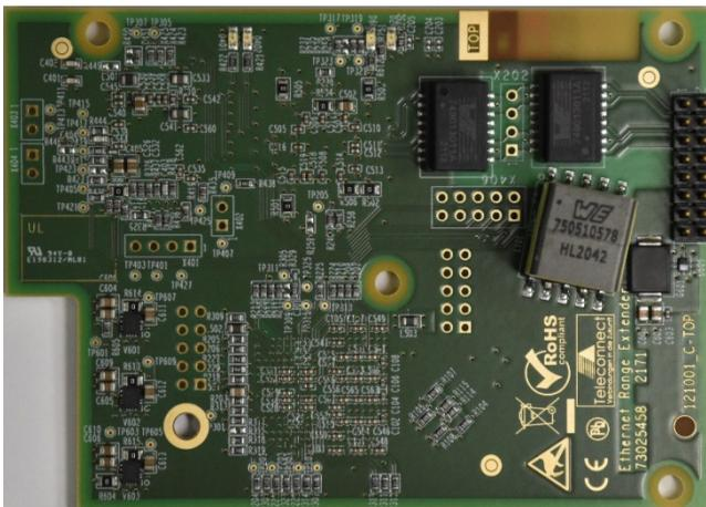
Fig. 5-1: Optional communication module
