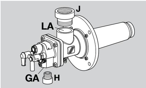
→ **BIC 125, BIC 140, BICW:** weld flange **K** to air pipe **P** for air connection **LA** and use NPT thread adapter **H** for gas connection **GA**.
