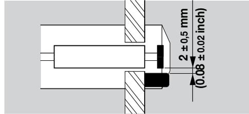
6 When the furnace chamber has cooled down, check the burner tube and burner block through the furnace flange.
