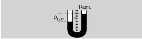
→ **Burners with gas measuring orifice:** set the differential pressure  $\Delta p_{\text{gas}}$  using the gas restrictor or via the integrated flow adjustment.
