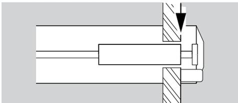
→ Distance of spark electrode from ground pin or gas nozzle:  $2 \pm 0.5 \text{ mm}$  ( $0.08 \pm 0.02''$ ).
