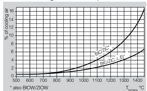
→ Diagram: the cooling air percentage specified in the diagram refers to the operating flow rate for air.
