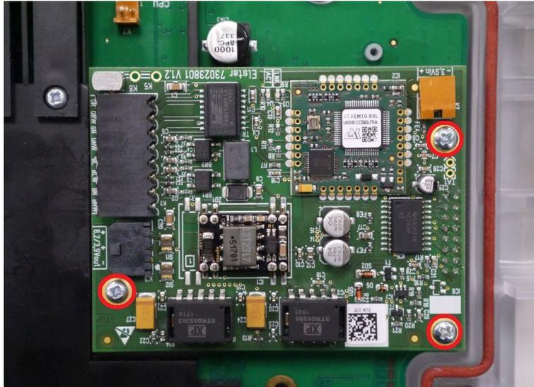
Once you have installed the Ethernet module in the DL230
