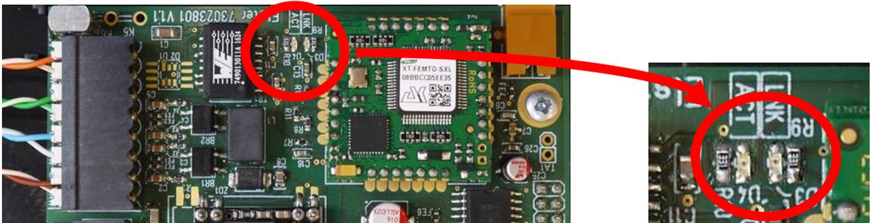
If the LEDs do not flash, either the module is not active (possible cause: the time window is still open) or there is a fault in the wiring.
