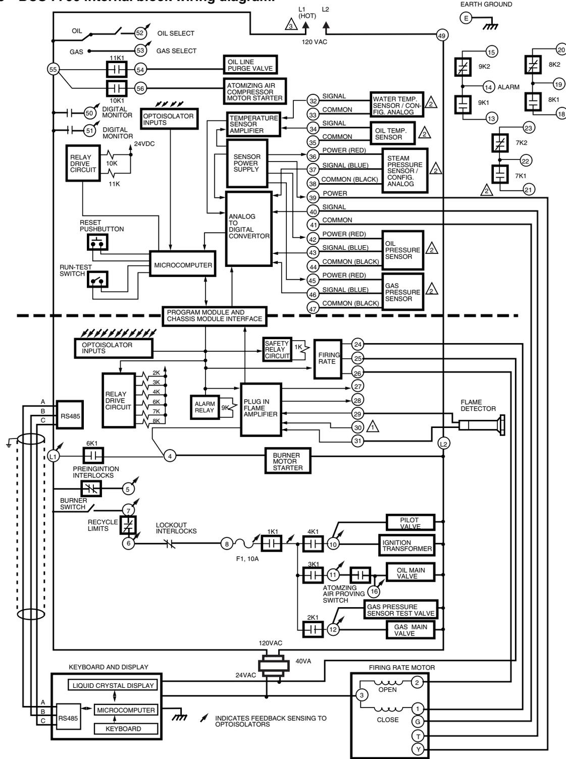
1 WIRING SHOWN FOR INFRARED FLAME DETECTOR FOR C7027
