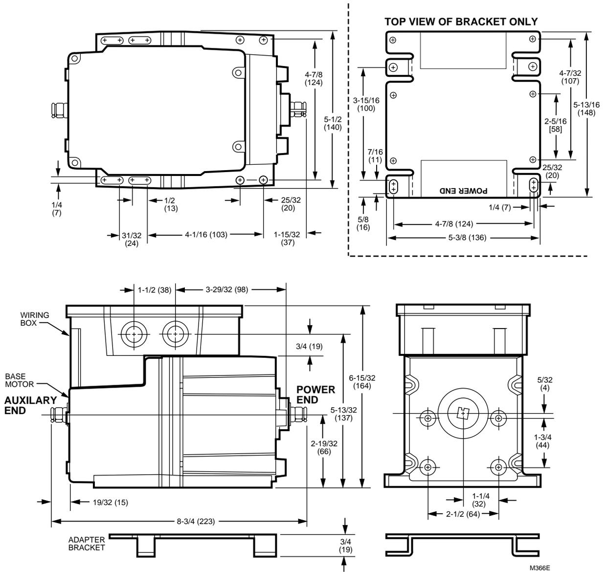
**Fig. 1. Dimensions of M7185, M7186 motors in in. (mm).
