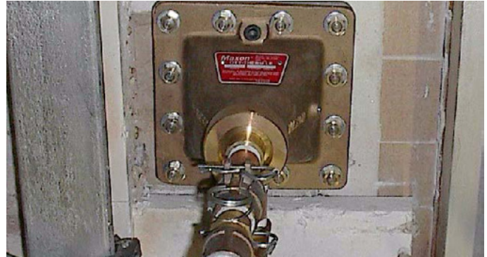
OXY-THERM LE mounted on a glass furnace
