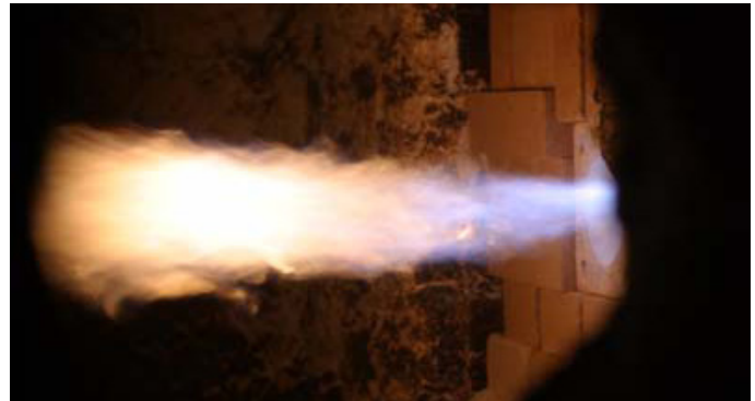
OXY-THERM LE staged flame pattern
