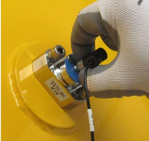
Figure 4: Disconnecting transducers
