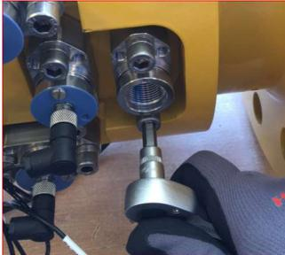
4. Screw the spindle into the bracket till the end
