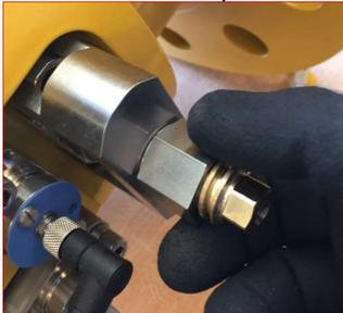
6. Use wrench SW 24 and spin the nut until the bracket is released
