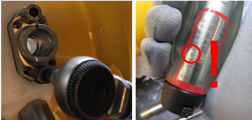
Figure 21: tightening the transducer mounting bolts to 8 Nm
