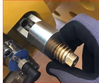
5. Attach nut to the spindle
