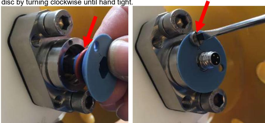
Figure 27: reinstalling the alignment disc and bolt
