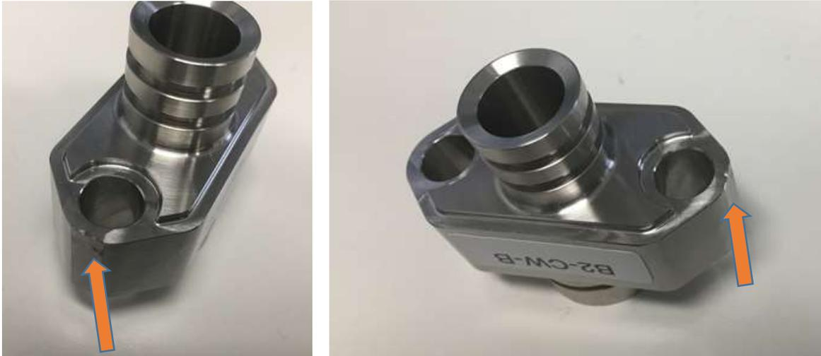
Figure 16. Marking sign on re-machined old bracket
