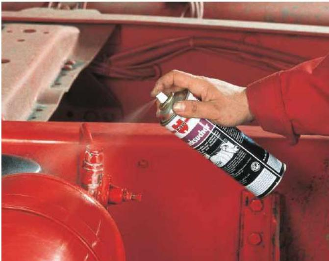
Figure 38. Gas leak detection agent
