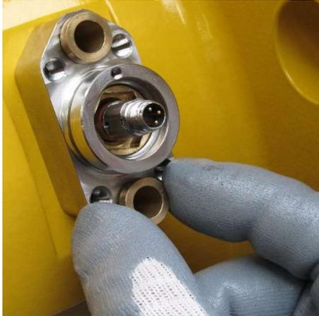
Figure 10: Removing the rivets
