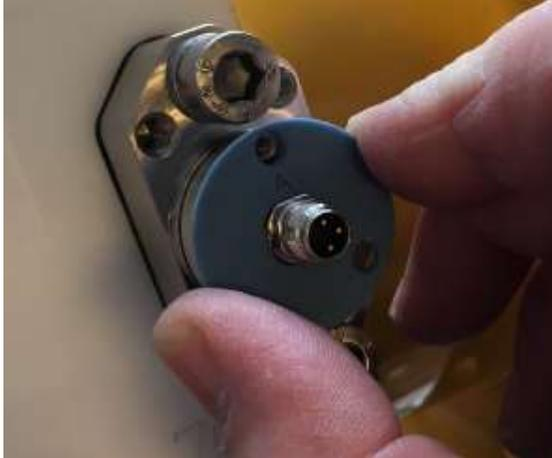
Figure 24: aligning the transducer
