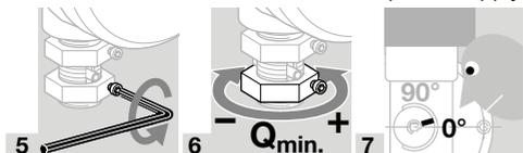
8 Once the settings have been adjusted successfully, retighten both screws to secure the adjusting nuts for  $Q_{min.}$  and  $Q_{max.}$ .
