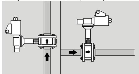
→ Installation in the vertical position with the direction of flow from bottom to top prevents condensation and dirt from accumulating on the stop bar of the butterfly valve.
