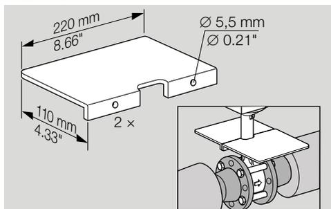
In conjunction with the butterfly valve BVHM, the solenoid actuator can be used for hot air of: up to 250°C (480°F), up to 450°C (840°F) when heat deflectors are installed.
