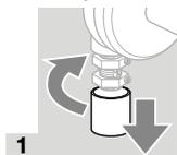
→ In order to set  $Q_{max.}$ , voltage must be applied to the solenoid actuator. The butterfly valve is closed when de-energized.
