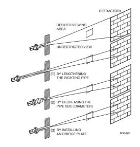
Fig. 2. Methods of reducing C7915A Detector field-of-view.
