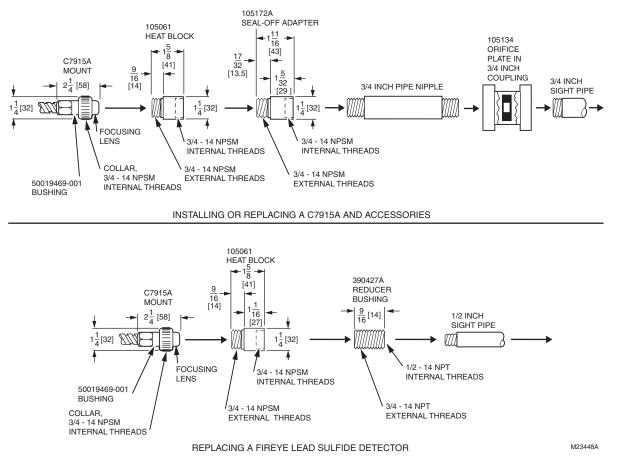
Fig. 1. Mounting dimensions of C7915A Infrared Flame Detector and accessories, in inches. (mm).
