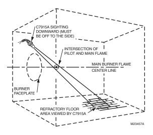
Fig. 6. C7915A Infrared Flame Detector aimed at floor of combustion chamber.
