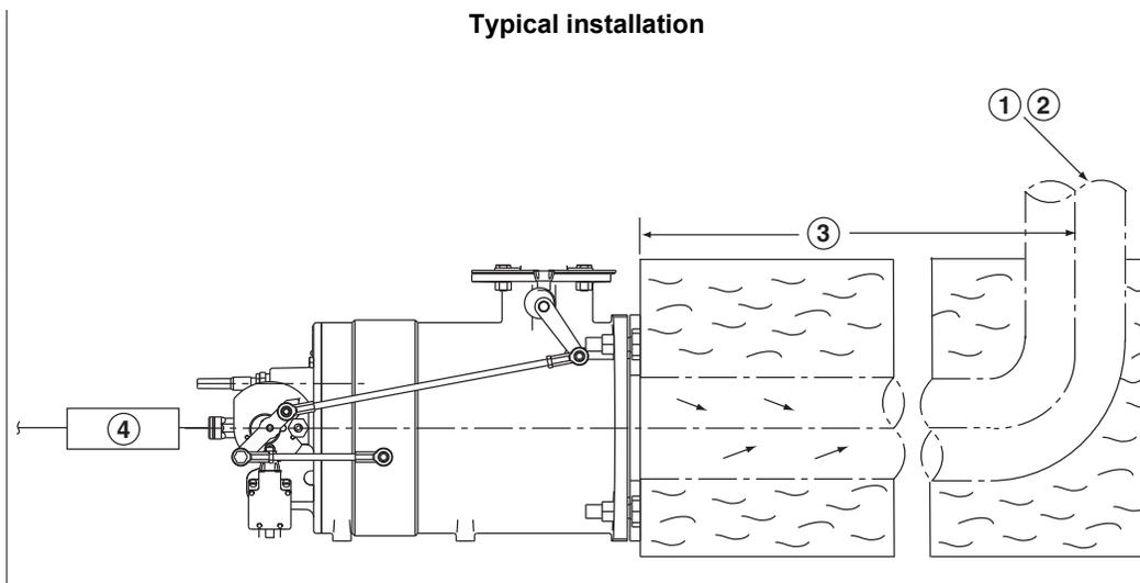
Small bore immersion tubes can be sized for efficiencies lower than 80% if tank space is limited or if complete freedom from tube condensation is desired.
