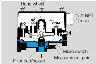
The pressure switch DL...ALT switches in the event of rising pressure.
