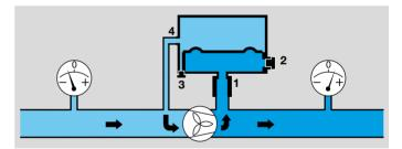
The higher absolute pressure is connected to port **1** (or **2**), and the lower absolute pressure to port **4** (or **3**). The remaining ports must be tightly plugged.
