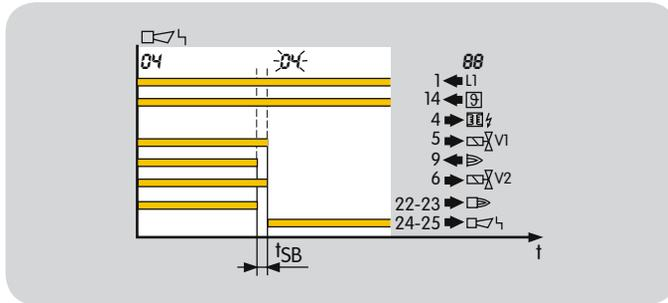
After a flame failure during operation, the IFD 450 will perform a fault lock-out within the safety time during operation  $t_{SB}$  (the safety time during operation  $t_{SB}$  is 1 second. The IFD 450 is available with a safety time of 2 seconds upon request). This involves closing the gas valves and disconnecting the power from the ignition transformer. The fault signalling contact closes and the display blinks and indicates  $\boxed{04}$  – see table “Program status and fault messages”.
