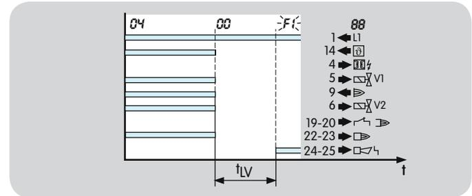
Flame simulation is signalled by at least one flame detector. The flame simulation delay time  $t_{LV}$  then starts to elapse. If the flame simulation is continued during the flame simulation delay time  $t_{LV}$  (max. 15 s), a fault lock-out will occur. The display blinks and indicates  $\square F \square$ .
