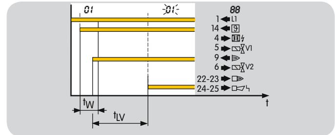
If flame simulation is signalled during start-up, the flame simulation delay time  $t_{LV}$  starts to elapse. If the flame simulation is discontinued during the flame simulation delay time  $t_{LV}$  (max. 15 s), the burner will start up. Otherwise, a fault lock-out occurs. The display blinks and indicates 02, see page 20 (Program status and fault messages).
