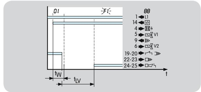
Flame simulation detected by at least one flame detector is signalled during start-up (no connection between terminals 19 and 20). The flame simulation delay time  $t_{LV}$  then starts to elapse. If the flame simulation is continued during the flame simulation delay time  $t_{LV}$  (max. 15 s), a fault lock-out will occur. The display blinks and indicates [Fl], see page 20 (Program status and fault messages).
