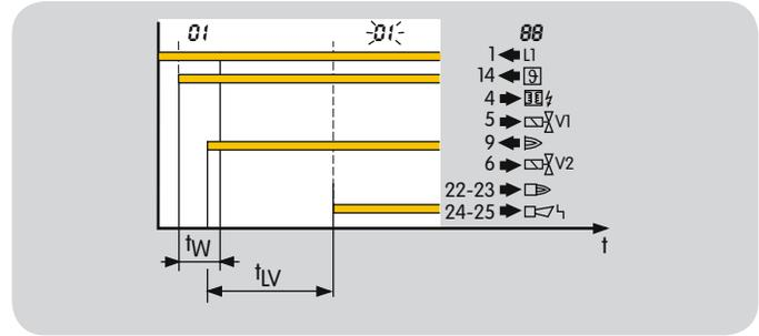
Flame simulation is an incorrect flame signal. If flame simulation is detected during start-up, the flame simulation delay time  $t_{LV}$  (max. 15 s) starts to elapse. If the flame simulation is discontinued during the flame simulation delay time  $t_{LV}$ , start-up can be initiated or operation continued. Otherwise, a fault lock-out occurs.
