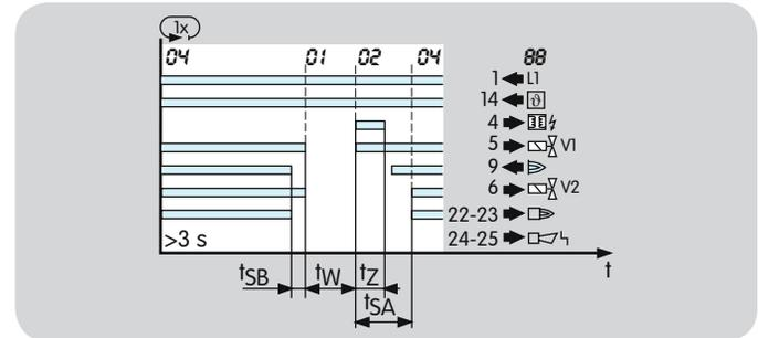
If the IFD 454 detects a flame failure after a minimum operating time of 3 seconds, the valves are closed and the operation signalling contact opened (terminals 22 to 23) within the safety time during operation  $t_{SB}$ .
