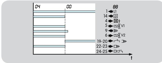
After switching off the start-up signal ( $\emptyset$ ), the valves close and the operation signalling contact (connection between terminals 22 and 23) opens. The burner switches off. The automatic burner control unit IFD checks in start-up position/standby, whether an extraneous signal (flame simulation) is present. The display indicates the current program status  $\square\square$ .
