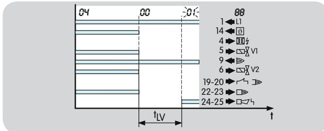
Once the burner has been shut down, flame simulation is signalled. The flame simulation delay time  $t_{LV}$  then starts to elapse. If the flame simulation is continued during the flame simulation delay time  $t_{LV}$  (max. 15 s), a fault lock-out will occur. The display blinks and indicates  $\square F \square$ .
