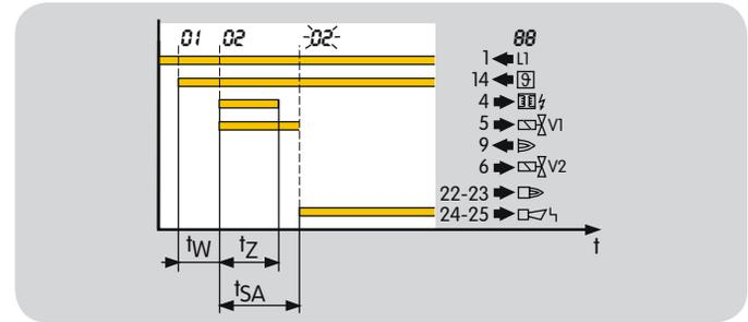
If, after a successful burner start, the automatic burner control unit does not detect a flame signal during the safety period on start-up  $t_{SA}$ , a fault lock-out will occur (fault signalling contact between terminals 24 and 25 closes). During the entire safety time on start-up  $t_{SA}$ , the pilot gas valve V1 is open. The display blinks and indicates 02, see page 20 (Program status and fault messages).
