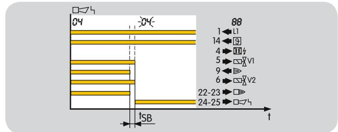
If the flame fails during operation, the valves are closed within the safety time  $t_{SB}$ .
