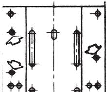
Mount with three short bolts and nuts at indicated holes.
