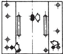
Mount with two short bolts and nuts and long bolt screwed into operator base through slotted hole.
