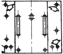
Mount with four short bolts and nuts at indicated holes.
