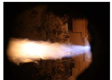
OXY-THERM<sup>®</sup> LE staged flame pattern
