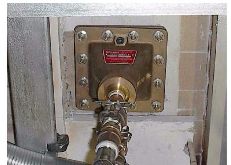
OXY-THERM<sup>®</sup> LE mounted on a glass furnace
