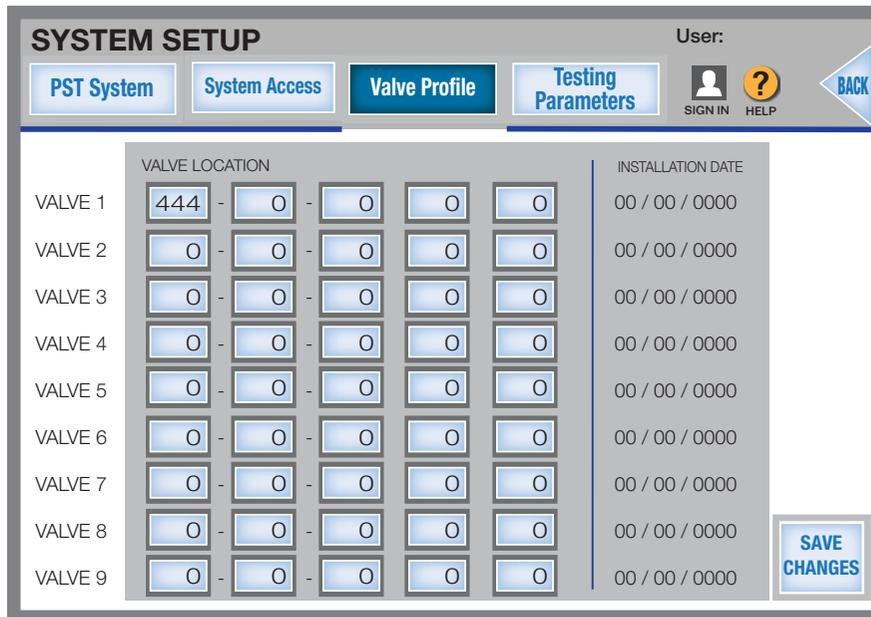
Lists the installation date for each valve in the system based on information entered on “PST System” screen during commissioning. Also provides the customer with the ability to set a custom numerical valve identifier (serial number, factory location, burner number, etc.) to help identify the valve’s physical location.
