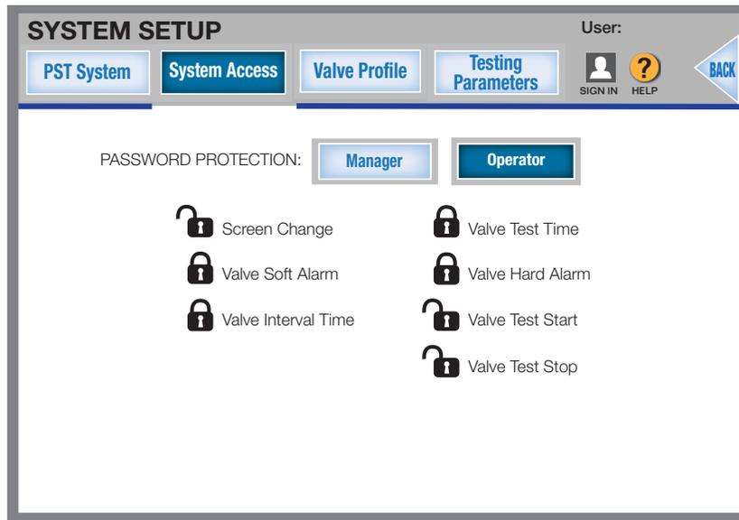
Visually indicates which users have the capability to perform or change various functions of the PSCHECK system, based on type of user (Manager or Operator). The permissions granted to Manager and Operator are factory-set and cannot be changed by the user.
