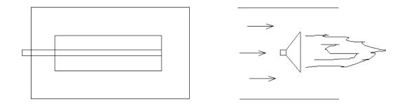
"HC" AIRFLO® burner in duct WITH profile plate
