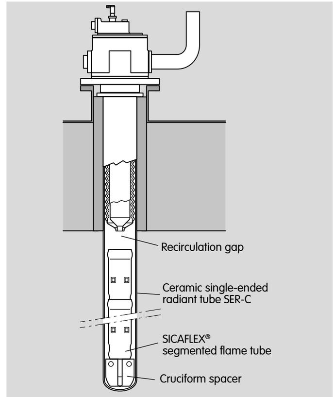
In vertically fitted single ended radiant tubes, a cruciform spacer ensures optimum sizing of the recirculation gap between the segmented flame tube and the burner, see page 9 (Cruciform spacer).
