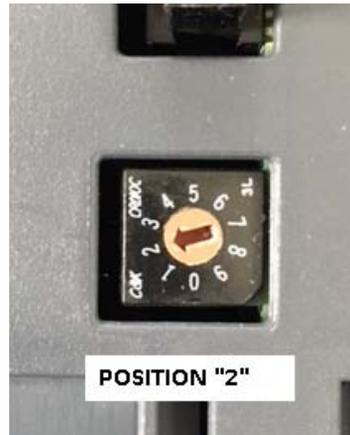
Amplifier Module Position Setting Switch
