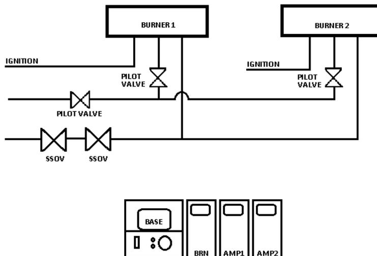
The dual-amplifier approach requires burner module configuration to support the feature as well as an additional physical setting on the amplifier module.
