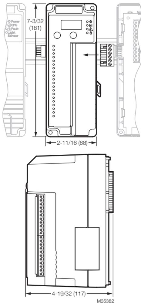
Fig. 1. Mounting dimensions of Digital I/O Module in in. (mm).
