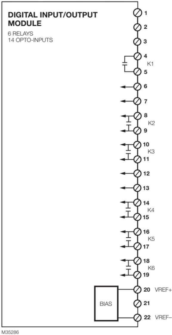
Fig. 3. Wiring diagram for limit control module.
