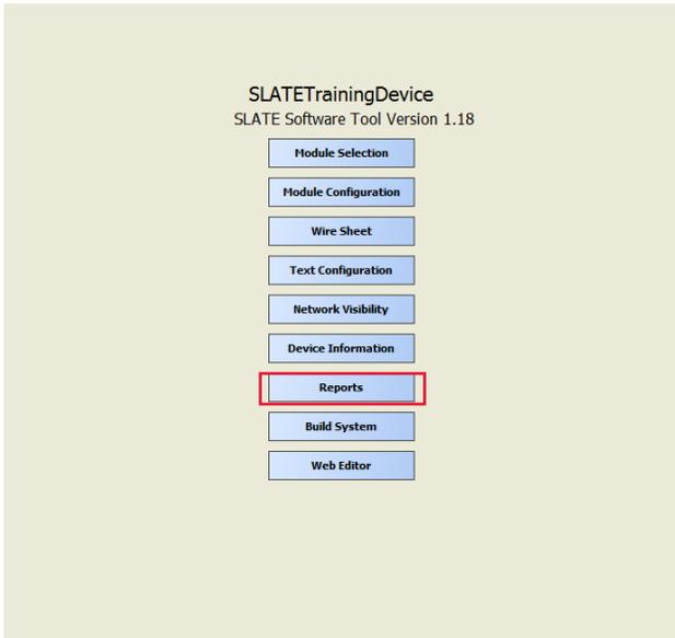
Reports can be generated identifying configurations an I/O usage, build errors, and communication interface for BACnet and Modbus.
