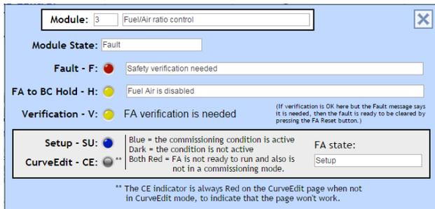
The Commissioning Section will be used to setup the actuators, the VFD, and do the curve edit. The gray area to the right of this
