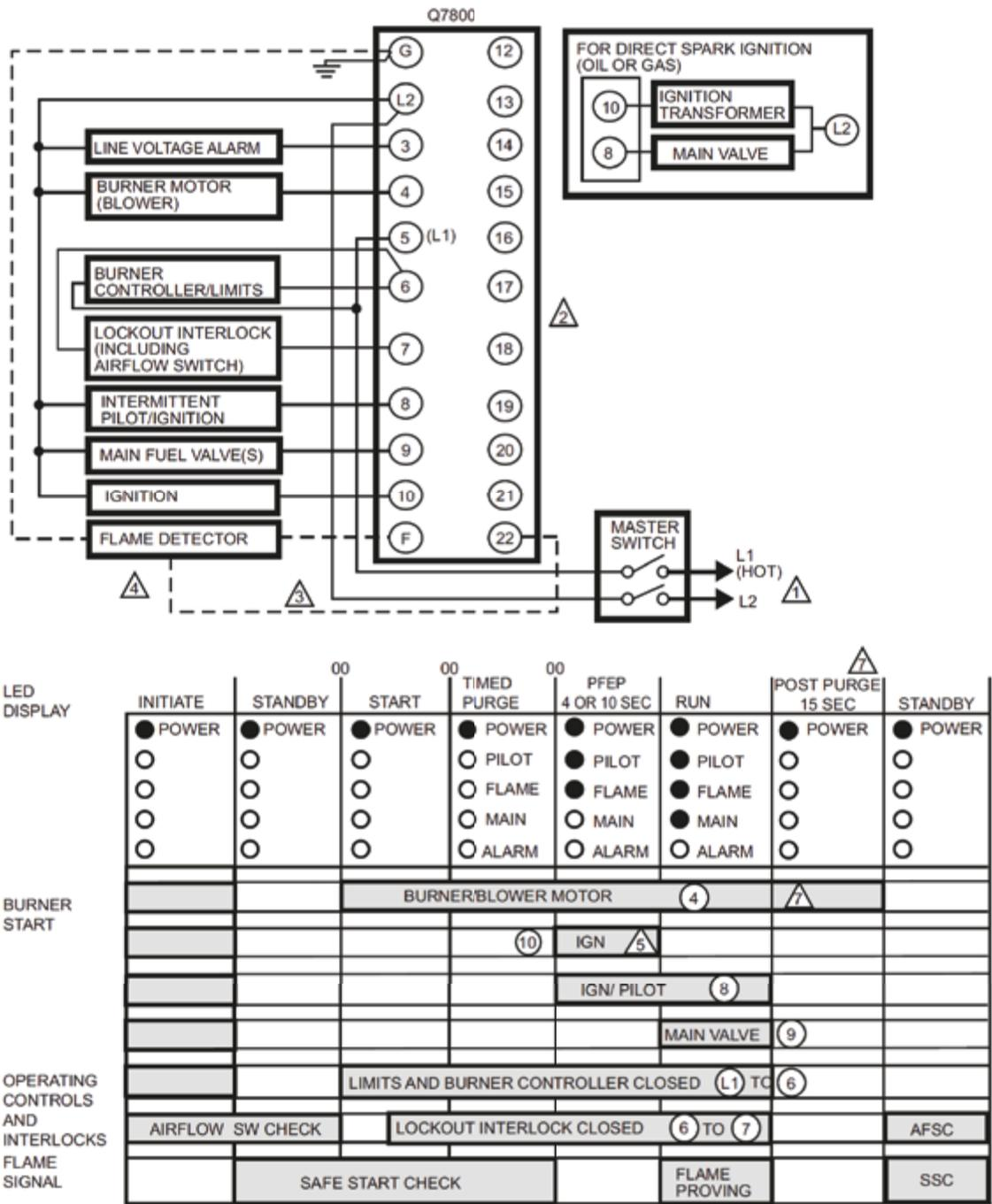
⚠️ RM7895, RM7896: 120 VAC , 50/60 HZ; EC7895: 220-240 VAC, 50/60 HZ POWER SUPPLY. PROVIDE DISCONNECT MEANS AND OVERLOAD PROTECTION AS REQUIRED.
