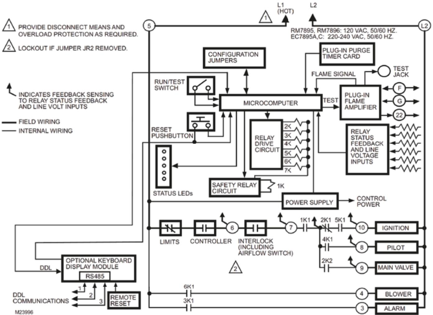
Fig. 1. RM7823 and EC7823 wiring for SIL 3 applications
