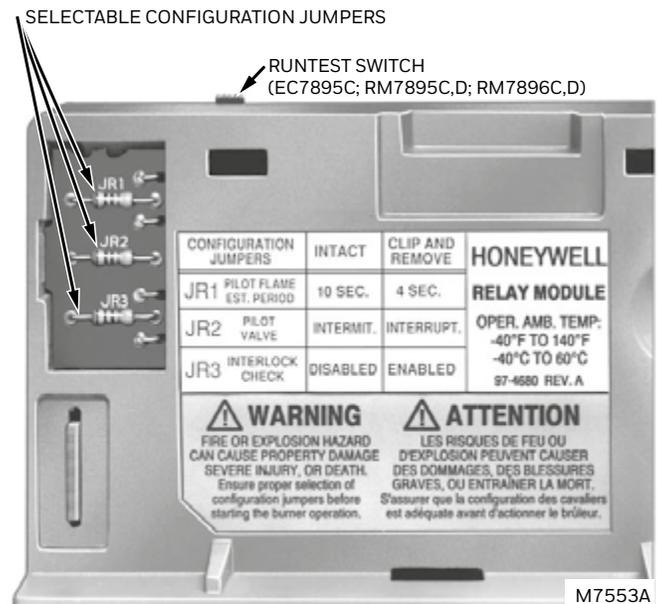
Fig. 6. Selectable site-configurable jumpers.
