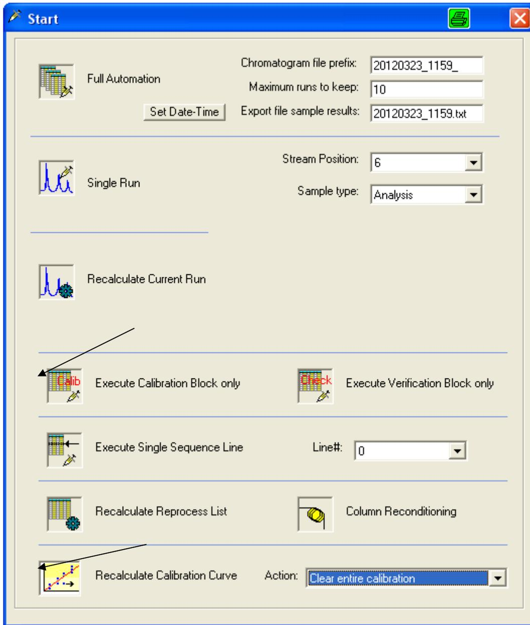
After the basic calibration is finished the option “initial calibration” in the menu method/ peak calibration should be deactivated and the option “calibration check” should be activated. This option becomes used for a check of the daily calibration.
