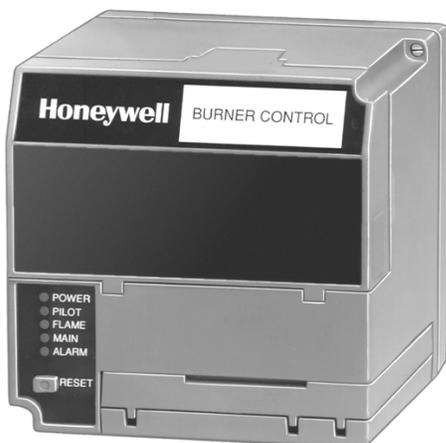
The RM7890, RM7895 provides on/off automatic burner sequencing, flame supervision, system status indication, system or self-diagnostics and troubleshooting. The RM7895 includes an output for the blower motor to provide purging.
