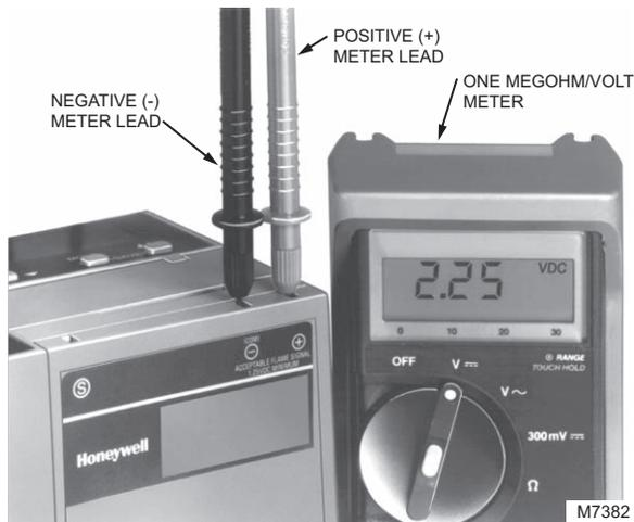
**Fig. 14. Flame signal measurement.**
