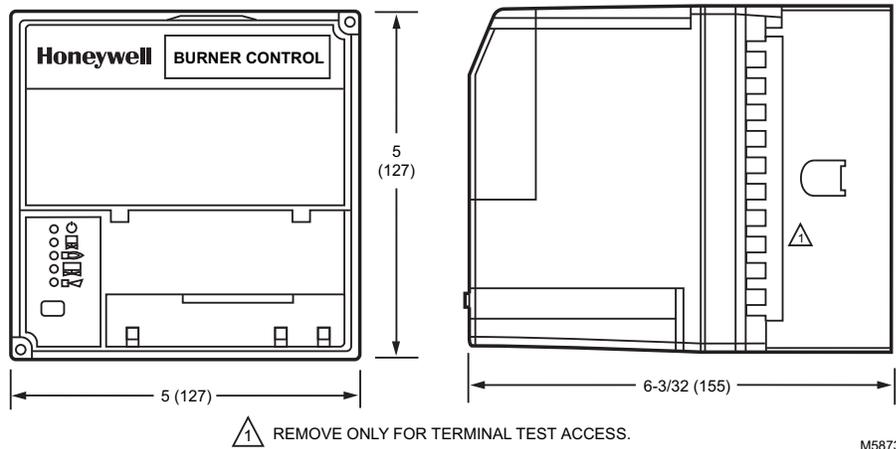
**Fig. 2. Mounting dimensions of RM7824A Relay Module and Q7800B Subbase in in. (mm).
