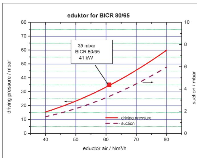
Fig. 6: Pressure profile at the BICR eductor
