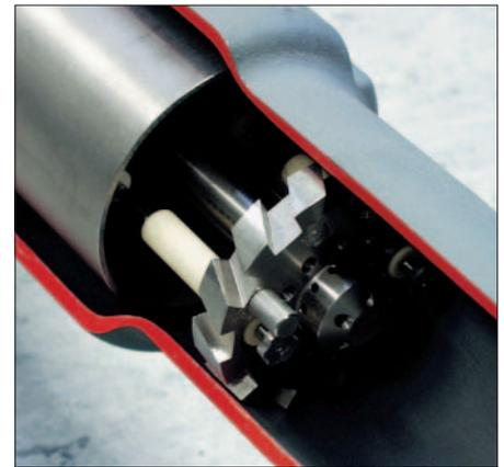
Fig. 3: Burner head in the SiC-tube
