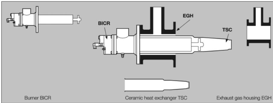
Fig. 1: Modular burner construction
