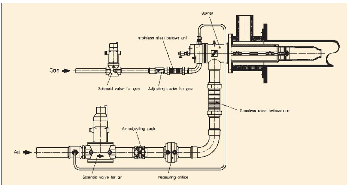
Fig. 4: Control of a BICR burner in the radiant tube
