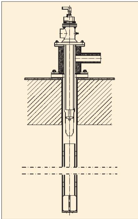
**Fig. 7:** BICR burner (21 kW capacity) installed in a previously electrically heated radiant tube.
