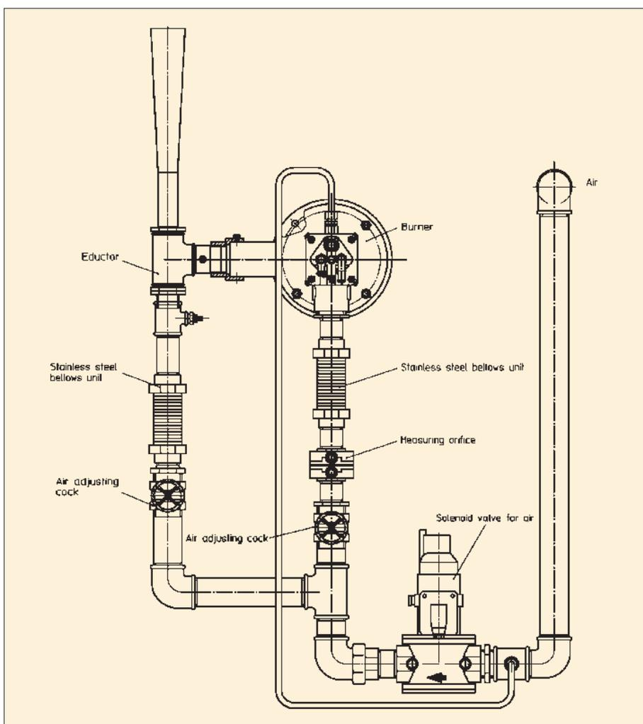
Fig. 5: Air supply for a BICR burner with eductor
