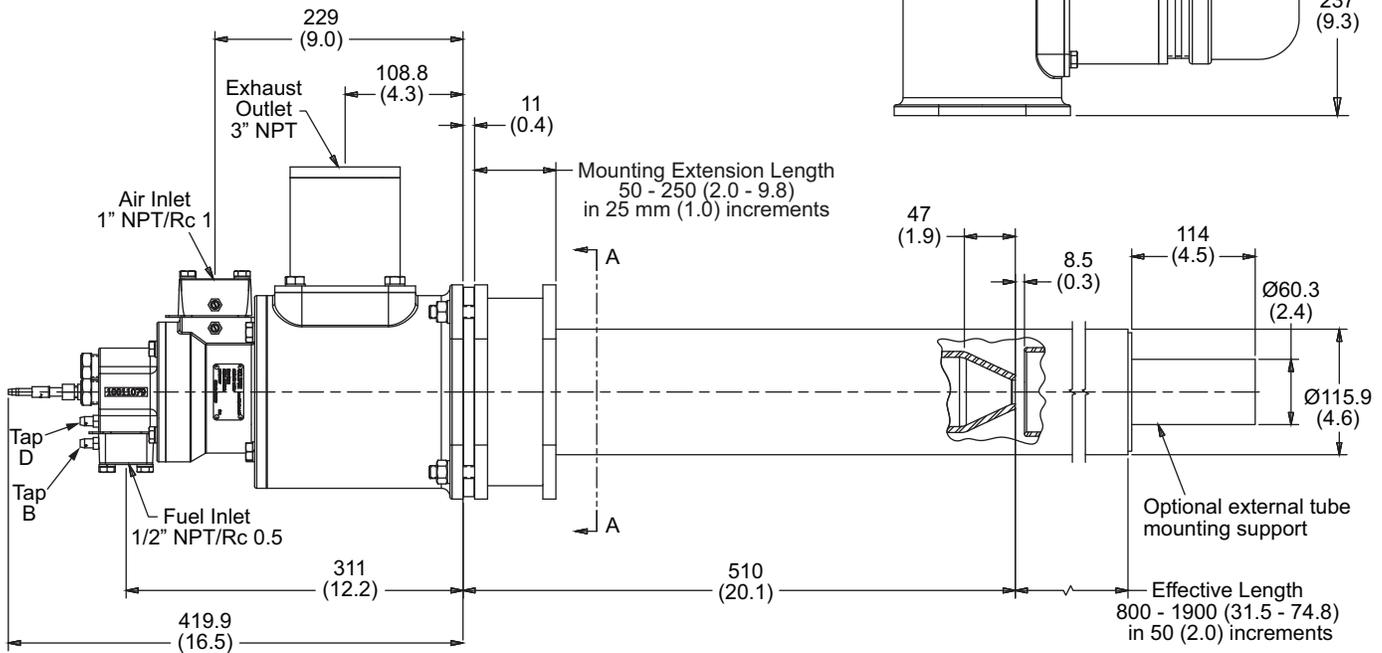
Version 5 outer tubes have a larger diameter flange than previous versions. Contact factory for retrofit of the burner to previous version outer tubes.
