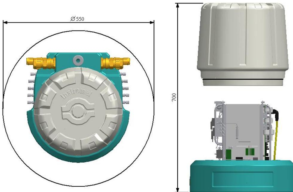
fig. 5-1 Mounting Dimensions and Installation Clearance
