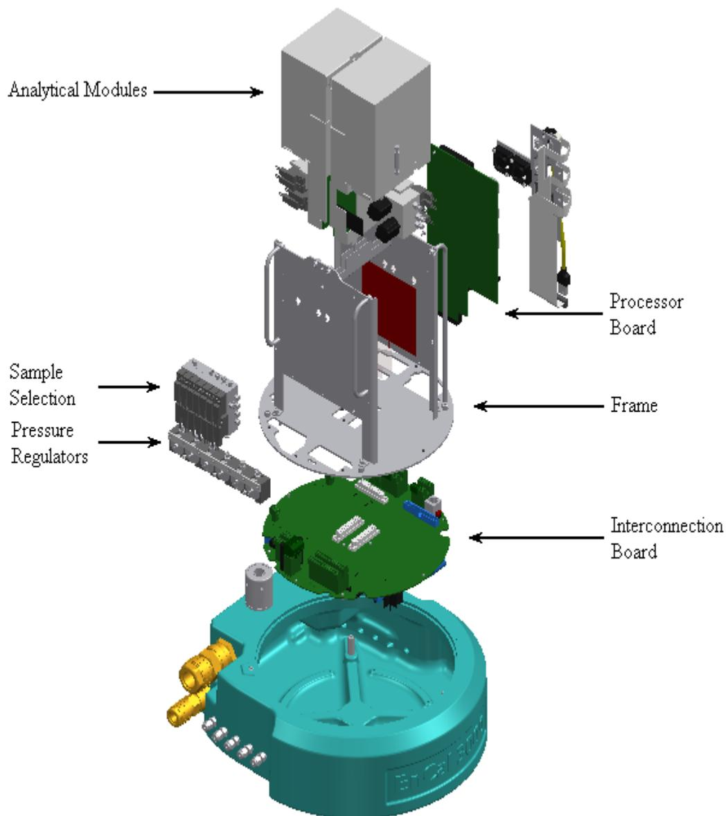
**fig. 2-1 Exploded View on the Internal Parts of the EnCal 3000**
