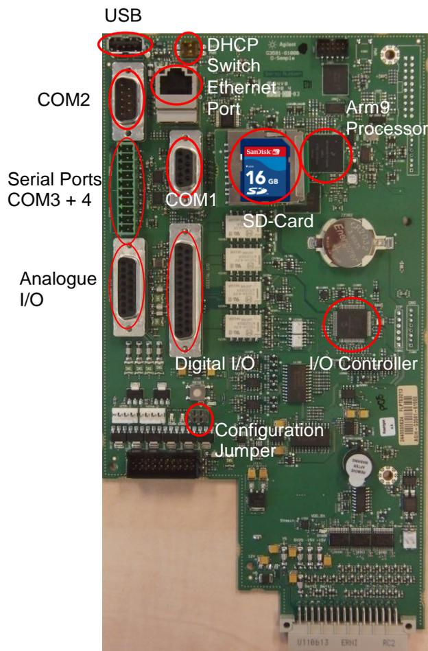
fig. 2-5: Processor Board connections
