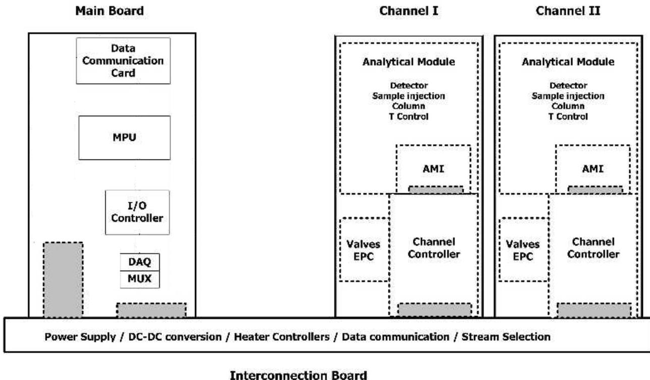
fig. 2-8 Overall Electrical Configuration of the EnCal 3000
