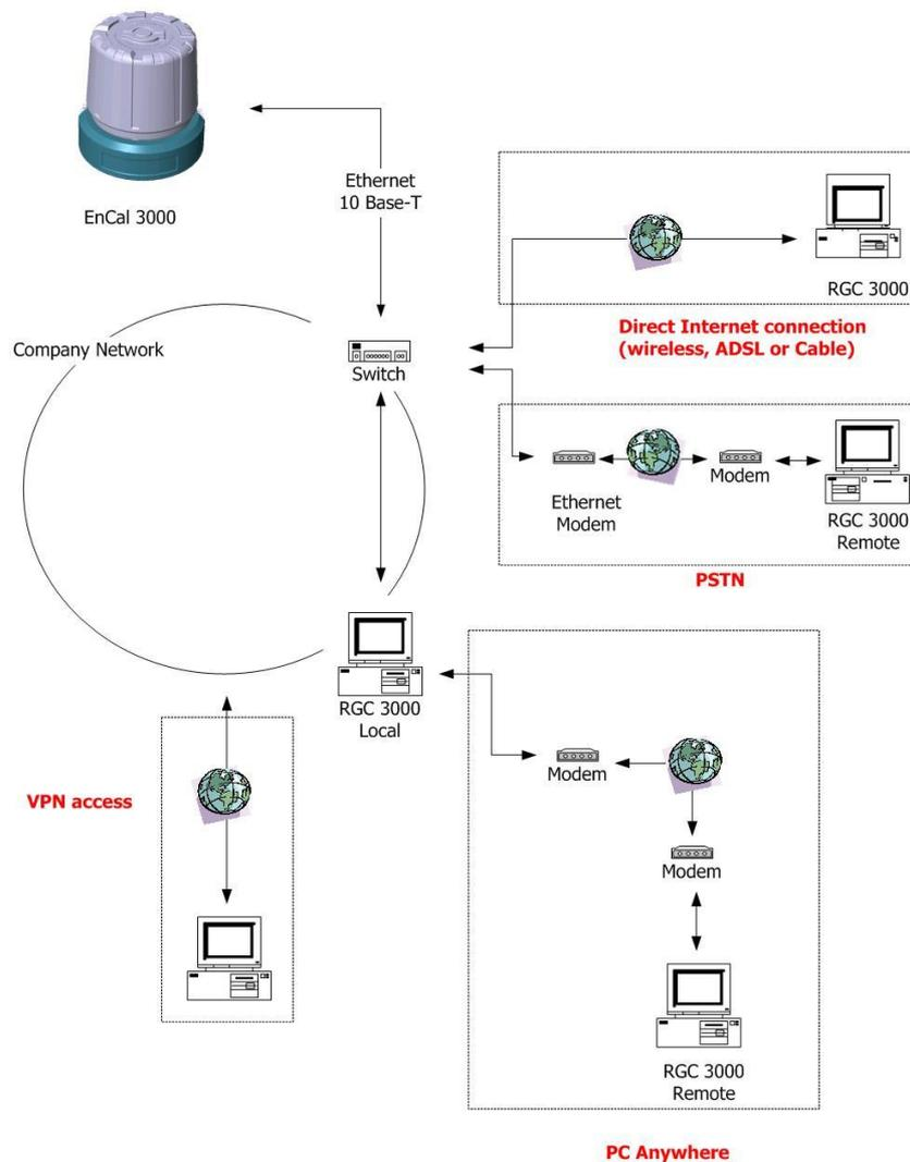
fig. 4-3 Remote Access to the EnCal 3000
