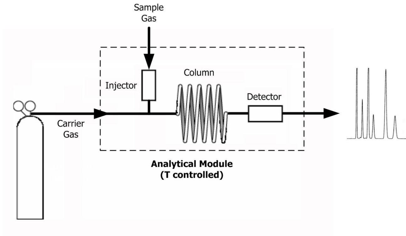
**fig. 1-1 Principle of a Gas Chromatography**
