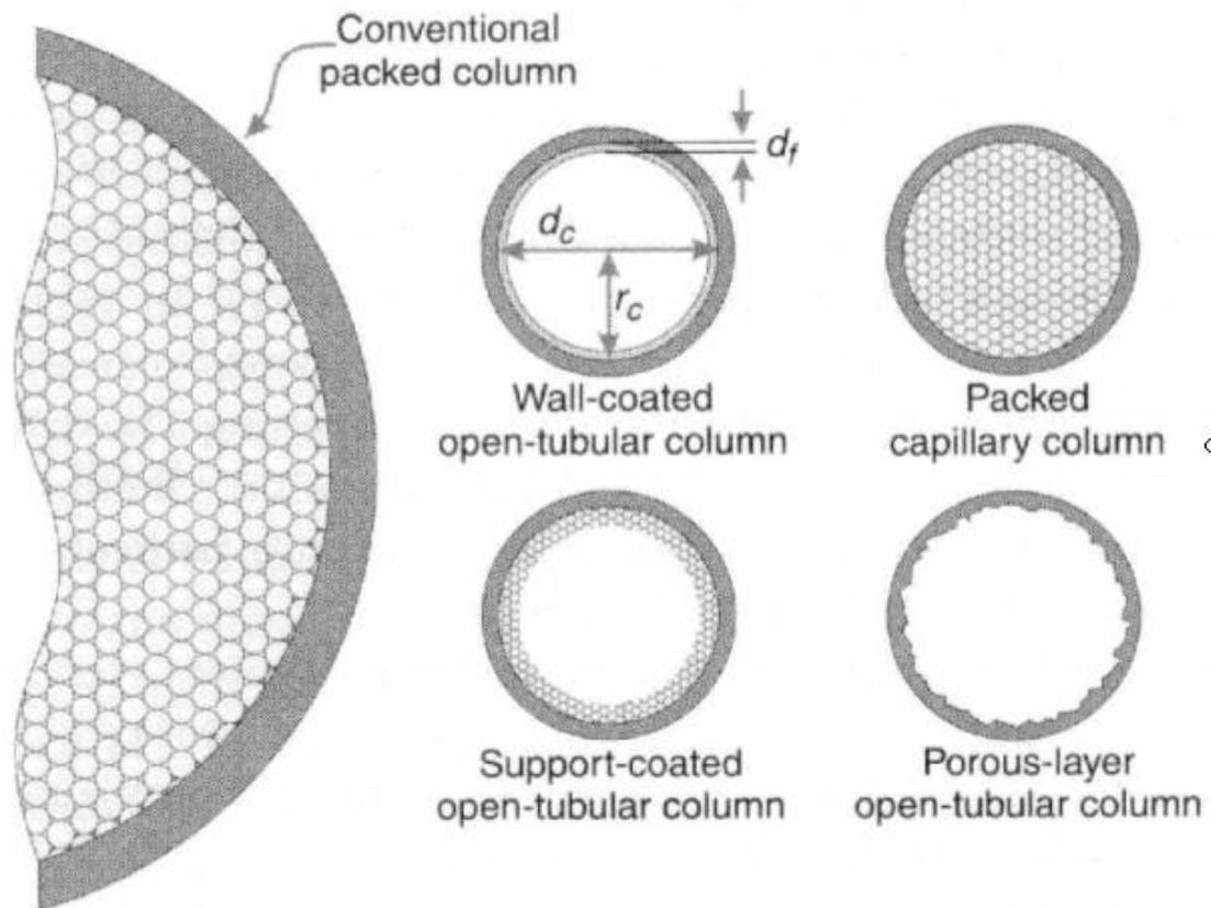
**fig. 1-2 Different types of gas chromatographic columns**
