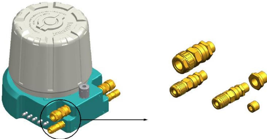
**fig. 2-14 Location of Cable Glands at the Back of the Enclosure Base**
