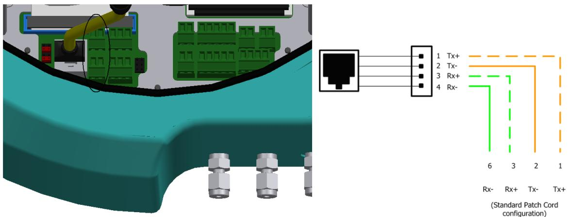
fig. 5-7 Location of Ethernet connector (J10) and wiring scheme
