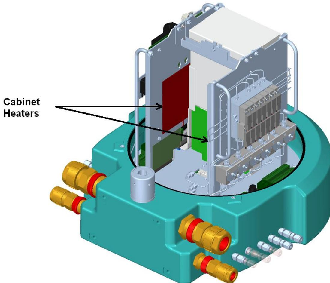
**fig. 2-9 Cabinet heaters location in the EnCal 3000**
