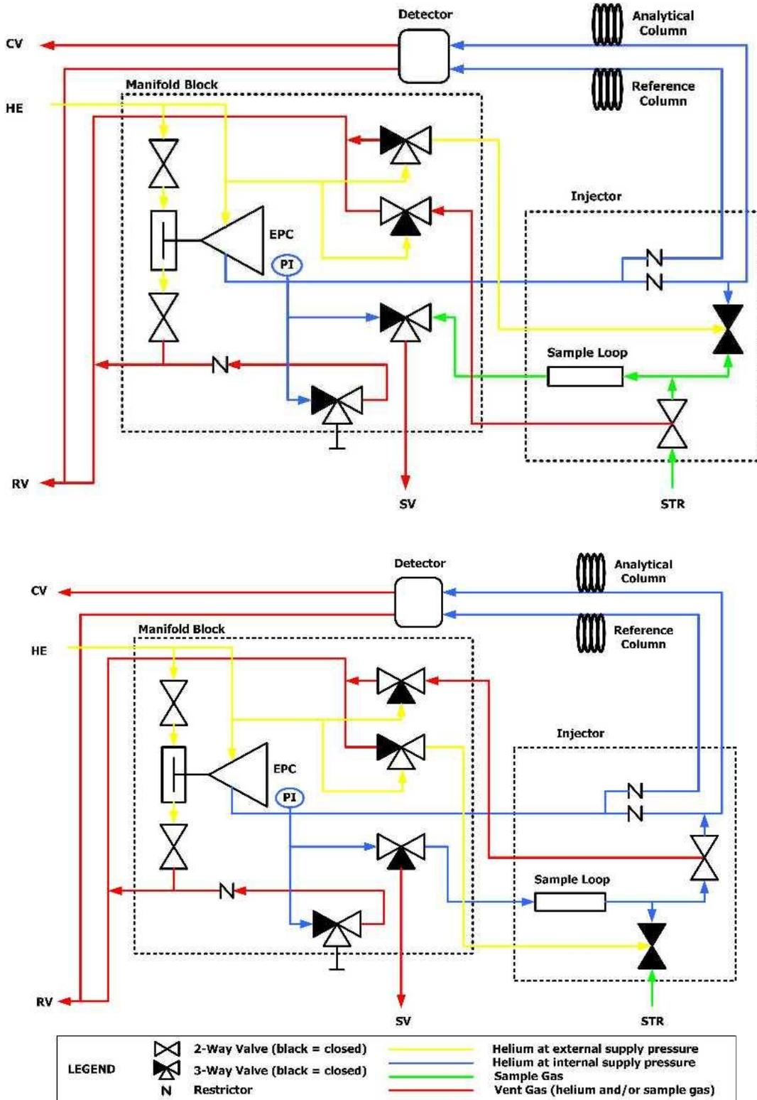
fig. 2-3 Internal Gas Flow Circuit for each Analytical Channel of the EnCal 3000, during Normal Operation (top) and sample Injection (below)
