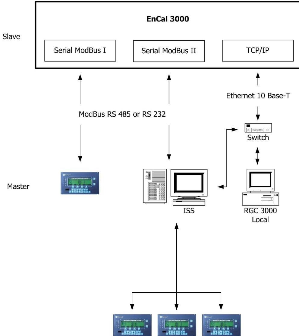
**fig. 4-2 Typical Data Communication Set-up for TCP/IP combined with Serial ModBus Communication with the EnCal 3000**
